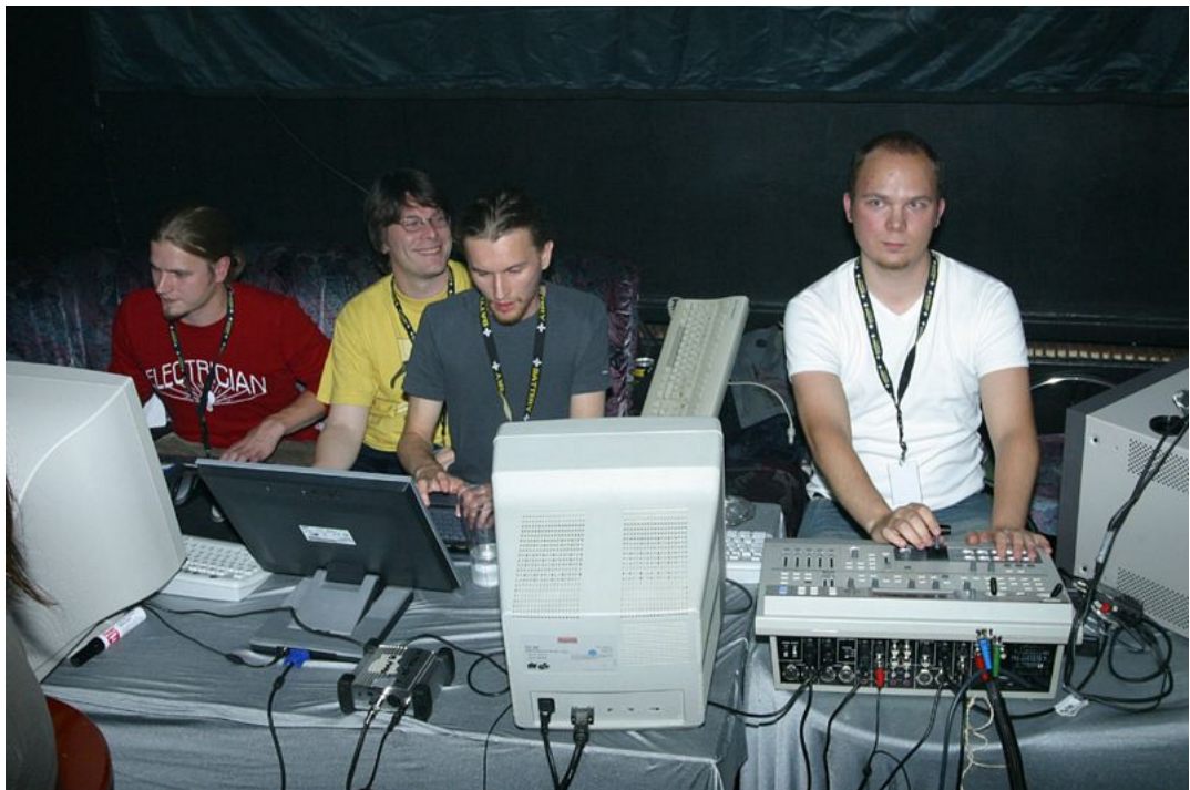
Figure 2. A more complex VJ set, where multiple computers are as video sources to a single video mixer. The system presented in this work is in actual use in the computer in the middle. (Photo (c) Heli Hintikka / http://www.pixheli.com/ )
